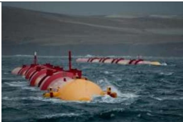
Pelamis Wave Power, Portugal: The Pelamis is an offshore wave energy converter that uses the motion of waves to generate electricity. The power is transmitted to shore using standard subsea cables.
