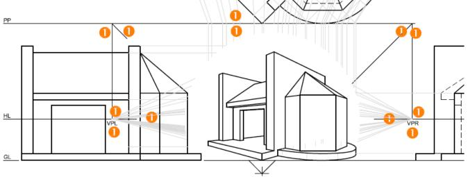
From the intersect on the PP a line is drawn perpendicular to the HL, the intersect on the HL is the vanishing point, LABEL the vanishing point LVP and RVP.
